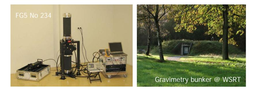
In 2007 the first measurements with a new absolute gravimeter purchased by TUD in 2006 at first order gravity stations were carried out. Also, continuous gravity measurements were carried out at Westerbork (IGS station).
